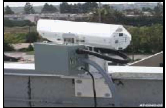
Figure 2.11: Angle Bracket Mounting (using JMP and M001)
